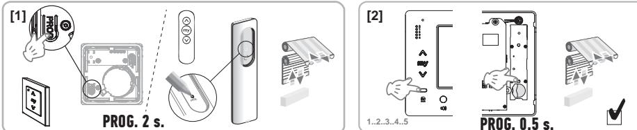
Note: To clear the monitor control programming on an io-homecontrol® receiver, repeat all the steps described above.
