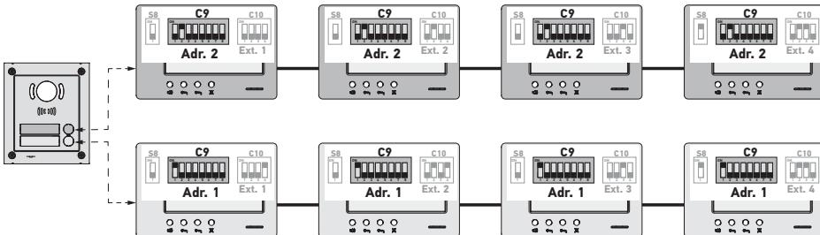
Note: if an external module with several call buttons is used (option available in 2017), the monitors must be configured with a different address for each house.
